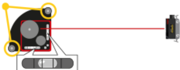
Rotate laser transmitter 180° and level the laser transmitter.
